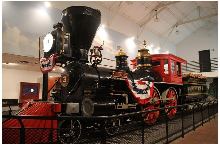
After the war ended, the *General* was repaired and continued service on the Western and Atlantic. In the 1870s, the *General* was completely rebuilt, it had received a new pilot, boiler, and other components. Most notably, its three dome configuration was reduced to two domes, and its Radley-Hunter style balloon stack was replaced with a diamond stack, as the engine had been converted to burn coal. Indeed, the rebuilt engine had little resemblance to its original form.
